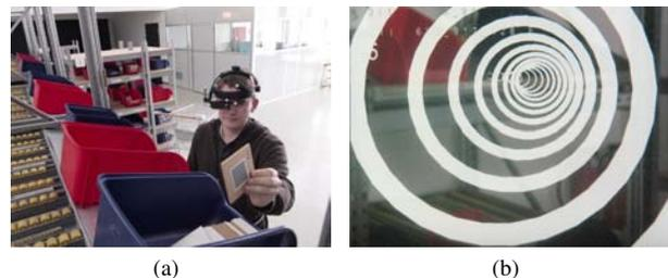
Figure 1: Current iteration of the AR system: Liteye HMD, infrared outside-in tracking, attention funnel navigation.
